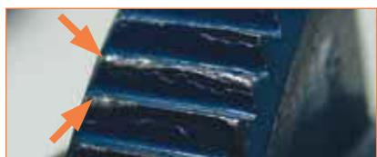
1 teeth damaged for 100% and 1 teeth damaged for 50%
