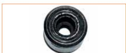
interior ring damaged for 100%
